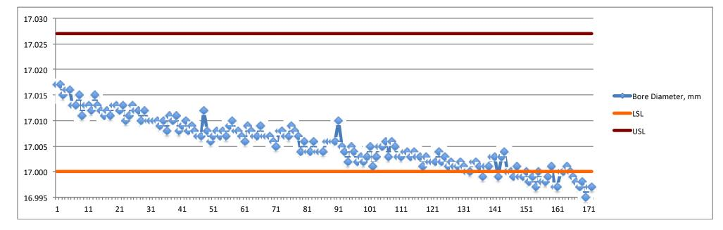
OBSERVATIONS of Parts manufactured at Hard Machining without taking Tool Wear Offset
