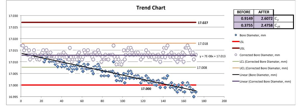
Simulation : Correction Factor (Offset) taken at every part based on the Gain ( $\beta$ ) and the Bias ( $\alpha$ ).
