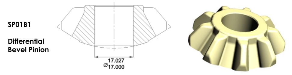
**Note**: Measurement done by an air-gauge, across the length of the bore, and the minimum of the measured value taken while making sure that the ovality and taper are below 3  $\mu$ , each.
